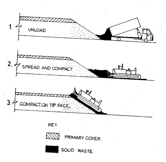
FIG. 3, FORMATION OF LAYERS-SOLID WASTE COMPACTED AND COVERED ON ALL EXPOSED SURFACES EACH DAY.
